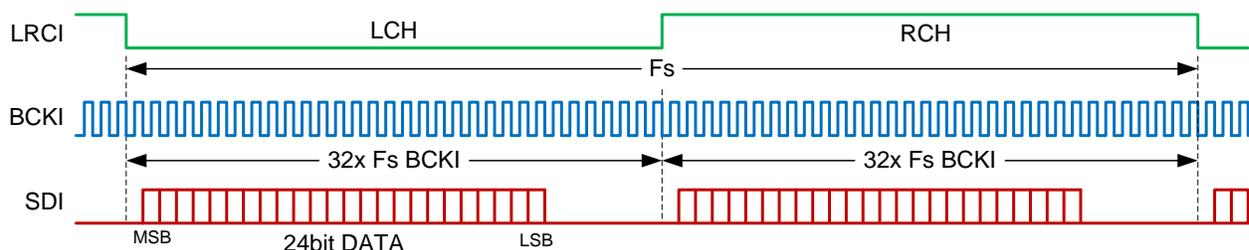
Figure 2. PT3344 Digital Interface Data Format (I<sup>2</sup>S)
