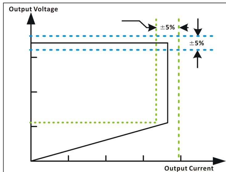
Fig.1 Typical CC/CV Curve
