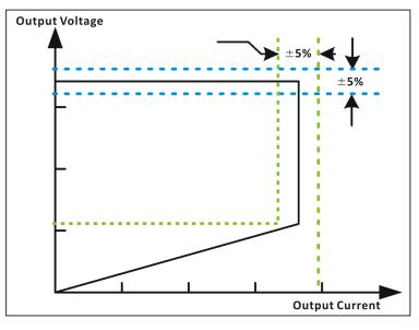
Fig.1 Typical CC/CV Curve
