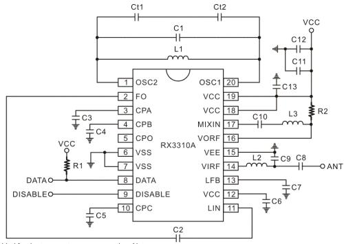
Note: Ct1, Ct2 are added for the temperature compensation. Not necessary.
