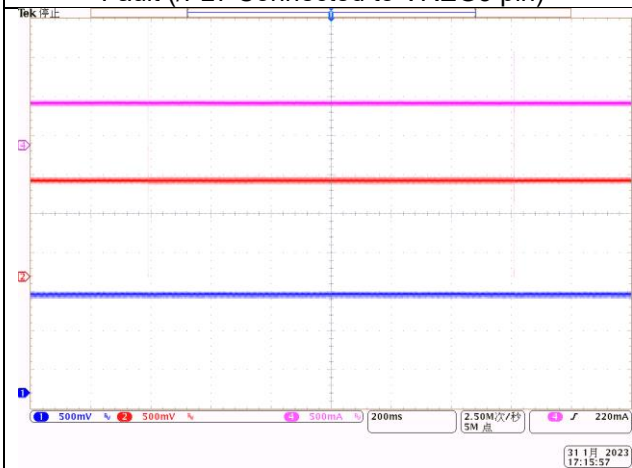
CH1: IADJ Voltage, CH2: IMON Voltage, CH4: Iout Time: 200 ms/div Figure 32. IMON Response to LED Short-Circuit Fault (/FLT Connected to VREG5 pin)
