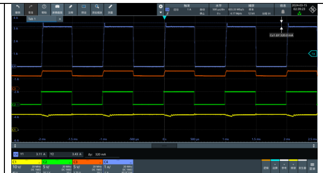
PWM Dimming ( D = 50\% , Frequency = 1kHz) CH1: V_{in} voltage; CH2: PWM input; CH3: LED+ to GND voltage; CH4: LED current
