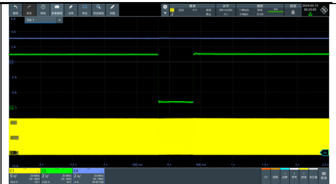
Output shorted (Vin=12V) CH1: SW pin voltage; CH2: Vout; CH4: Output Current;
