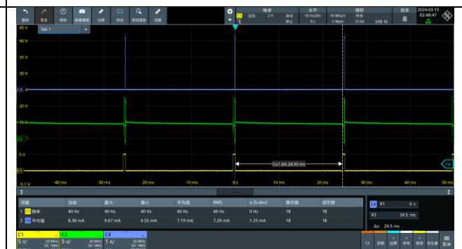
PWM Dimming ( D = 1\% , Frequency = 40Hz) CH1: PWM input; CH2: V_{sw} ; CH4: LED current
