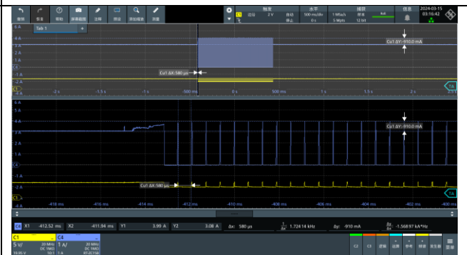
CS shorted to GND (Vin=12V) CH1: LED+ to GND voltage; CH4: LED Current;
