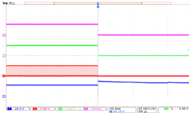
CH1: VCSP; CH2: GDRV; CH3: /FLT; CH4: ILED Time: 200ms/div Figure 60. SCP Operation (Normal → Short) DRL Mode
