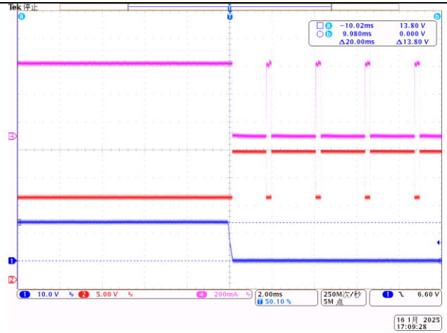
CH1: PWMI CH2: PDRV CH4: ILED Time: 2-ms/div Figure 25. DRL Mode → PWM Mode
