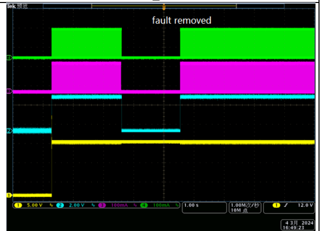
Open load in PWM mode (FAULT_A and FAULT_S floating) CH1=VIN/EN,CH2=FAULT_A,CH3=IOUT1,CH4=IOUT2
