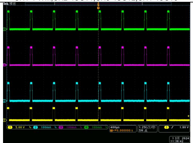
PWM Dimming, f_{PWM}=2\text{kHz} , D=10\% CH1=PWM,CH2=IOUT1,CH3=IOUT2,CH4=IOUT3
