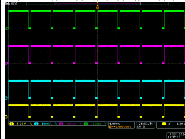
PWM Dimming, f_{PWM}=200\text{Hz} , D=90\% CH1=PWM,CH2=IOUT1,CH3=IOUT2,CH4=IOUT3
