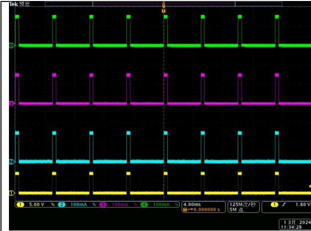
PWM Dimming, f_{PWM}=200\text{Hz} , D=10\% CH1=PWM,CH2=IOUT1,CH3=IOUT2,CH4=IOUT3
