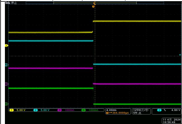
Open load Protection CH1=VOUT2,CH2=FAULT,CH3=IOUT2,CH4=IOUT1
