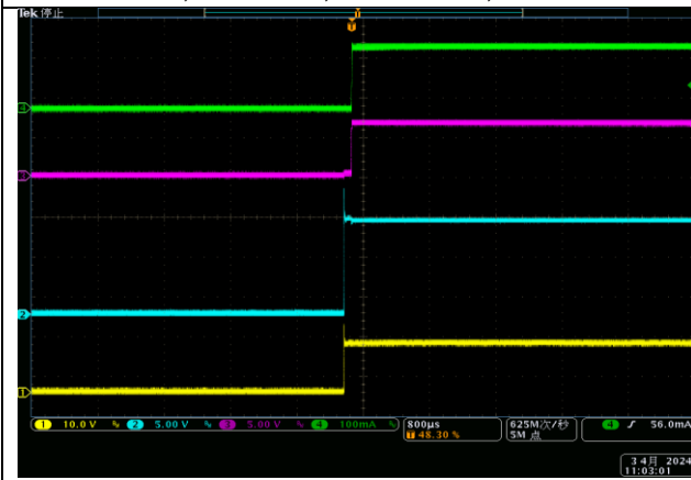
Fast Power-Up Waveform CH1=VIN,CH2=EN,CH3=VOUT1,CH4=IOUT1
