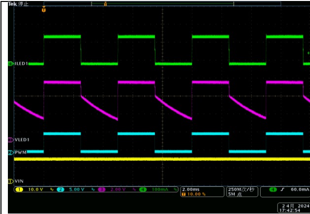
PWM Dimming, f_{PWM}=200\text{Hz} CH1=VIN,CH2=PWM,CH3=VOUT1,CH4=IOUT1
